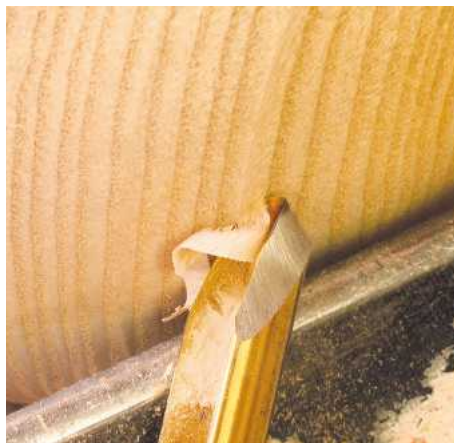
▲ Pic.8 This is how the shaving comes off the tool when you are turning with the long-grind bowl gouge in a pull cut. The shaving comes off the cutting edge and rolls around the flute before exiting
